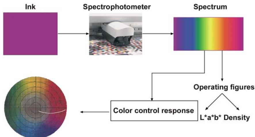
The colorimetric control process. Both the operating figures and color control response are derived directly from the spectrum of the measured ink.
