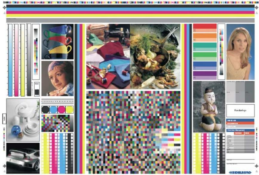
As well as the ECI\_2002 chart for profile creation, the Heidelberg Color Calibration Test Form also contains elements for determining the printing characteristics, ink trapping, ink fading, zonal ink distribution and images for optical judgement.
