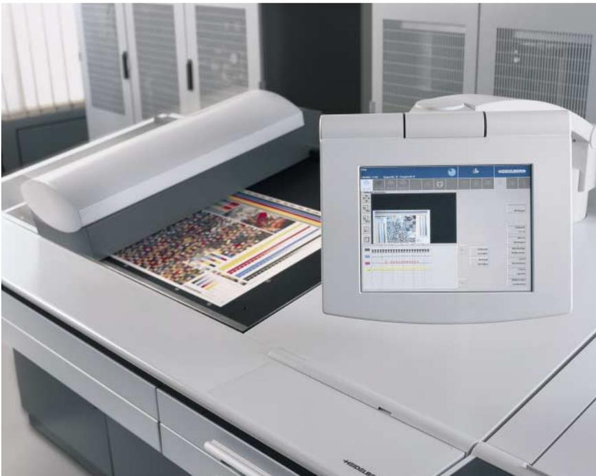
Prinect Image Control performs spectrophotometric measurement of the entire print image. Up to 4 Speedmaster® presses can be connected.
