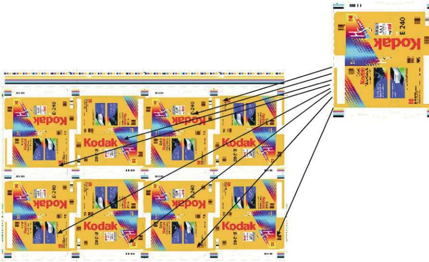
The values of an individual copy can be transferred as a reference to the entire print sheet. A copy from a fresh print sheet or a sample copy can be used for this purpose.
