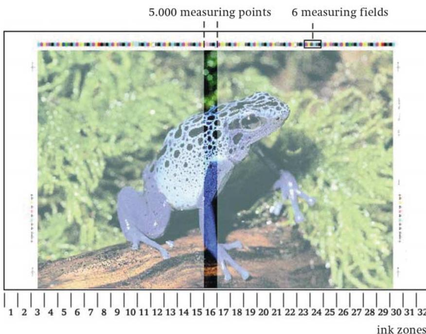
Prinect Image Control provides up to 5000 measuring points for each ink zone during image measurement. In contrast, only 6 measuring fields are evaluated during color bar control.
